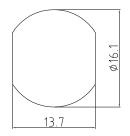
RECOMMENDED MOUNTING HOLE MAX. PANEL THICKNESS: 4.2MM TOLERANCE: ±0.07
