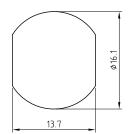
RECOMMENDED MOUNTING HOLE MAX. PANEL THICKNESS: 9MM TOLERANCE: ±0.07
